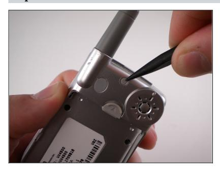
Remove the rubber grommet using a Spudger.
