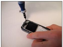
Remove the six screws with a T-6 Torx screwdriver.
