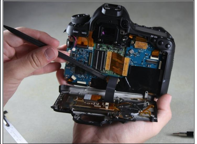
**⚠️ A black ribbon wire connects the rear panel to the inside of the camera. Breaking this wire would make your rear screen and buttons non-functional.**
