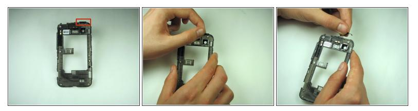
Firmly grasp the power button, located on the upper right corner of the mid panel, and gently lift it up and off the mid panel.
