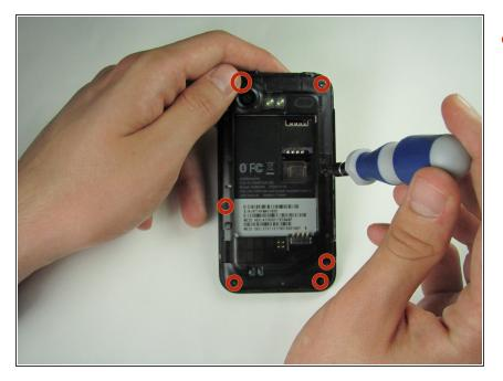
Remove the seven 1.42 mm Torx T5 screws
