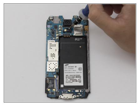
• Remove the single silver 4 mm screw from below the rear camera with a Phillips#00 screw driver.
