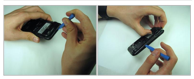
• Use a plastic opening tool to run along the phone's side and lever mid panel upward.
