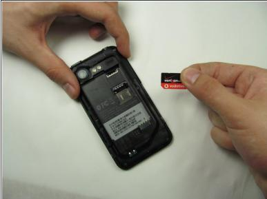
Keep sliding SIM card until completely free from holding apparatus. Now remove the SIM card.
