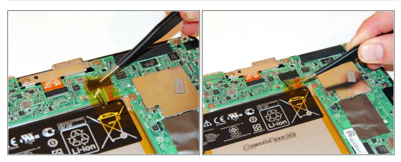
Gently pull back the yellow transparent plastic covering on top of the battery connection port.
