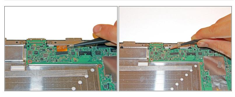
At the top end of the motherboard, use tweezers to gently slide the orange connection apparatus out of the connection port.
