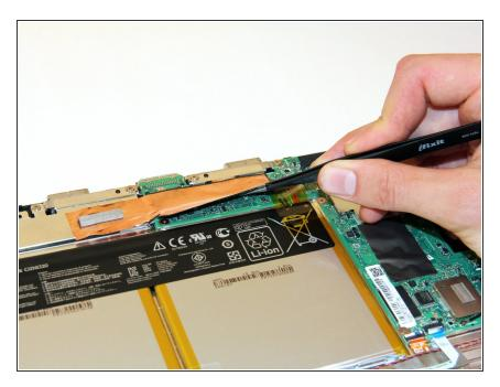
Remove the copper tape carefully.
