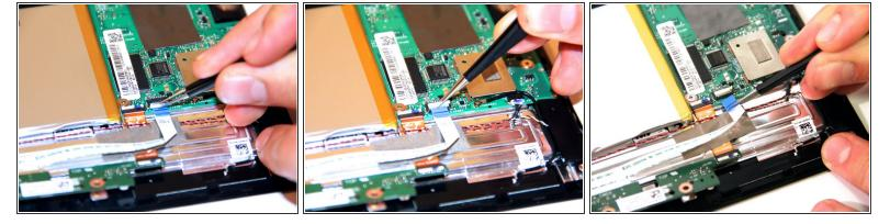
• Lift up the power button cable retention clip on the motherboard and pull the cable out.
