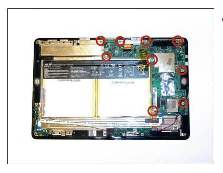
Remove the marked screws by using a Phillips #1 screwdriver.
