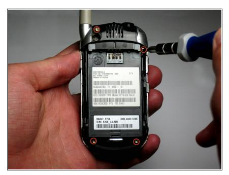
Use a Torx T6 screwdriver to remove the 4 screws that secure the back plate of the phone.
