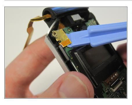
Use a plastic opening tool to peel off the gold tape that holds the flex cable in place.
