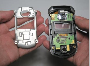
Remove the four screws holding in the metal cover.
