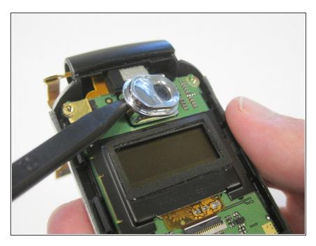
Use a spudger to remove the plastic protector case around the camera.
