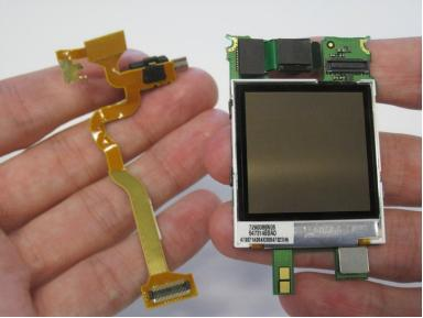
Use a spudger to detach the ribbon cable from the motherboard.
