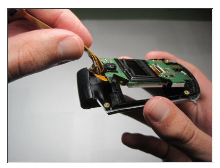
Remove the ribbon cable and the motherboard (still connected) from the frame of the phone.
