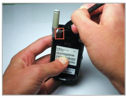
Use a spudger to remove the rubber plug from the upper left corner of the back of the phone.
