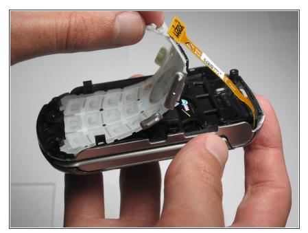
Remove the keypad from the bottom half of the phone.
