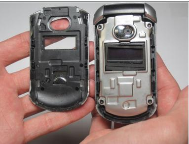
Use a plastic opening tool to remove the front cover of the phone.
