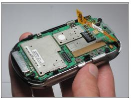
• Use a spudger to remove the ribbon cable from the motherboard.
