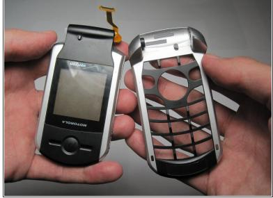
Slide the ribbon cable through the rectangular hole in the bottom half of the frame.
