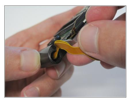
Slide the ribbon cable through the tiny slit located in the hole on the side of the frame.
