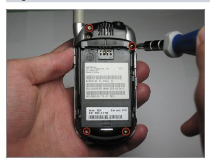
Using a Hex T6 screwdriver, remove the 4 screws holding the back plate of the phone in place
