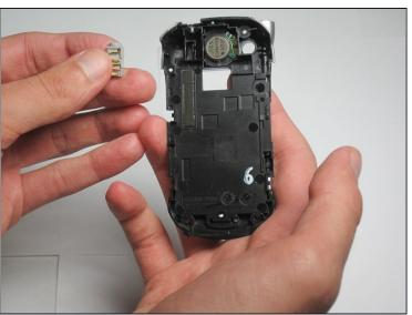
On the back casing, using a spudger, push into the headphone jack at an upward angle to pop it out
