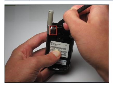
Use Spudger to remove rubber plug from upper left corner of the back of the phone
