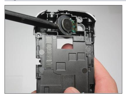
Using a spudger, remove the speaker
