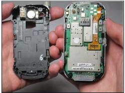
• Using your hands, pull up on the back plate while pulling on the 3 side tabs to remove the back plate.
