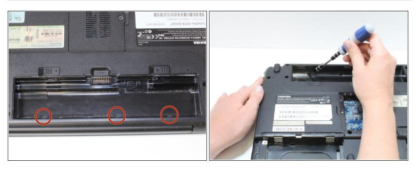
Remove the three 3mm Phillips #1 screws inside the battery compartment.
