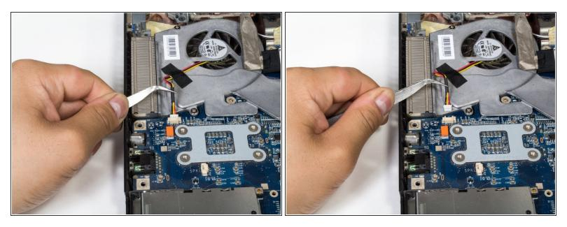
• Using tweezers, disconnect power cable by gently pulling white end straight away from its socket.
