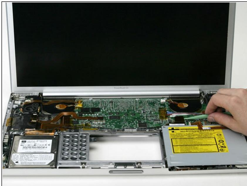
**⚠** The optical drive ribbon cable is very fragile. Be sure to gently lift up the cable on the sides. Do not lift up on the cable from the end closest to the display.
