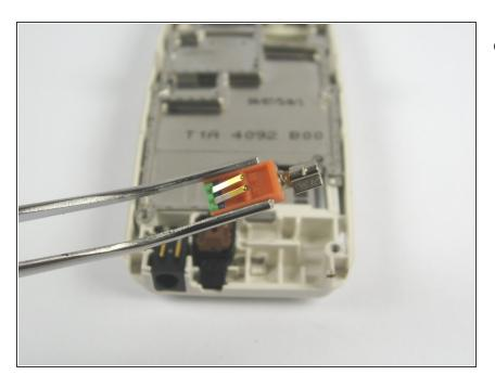
The vibrating unit is now removed.
