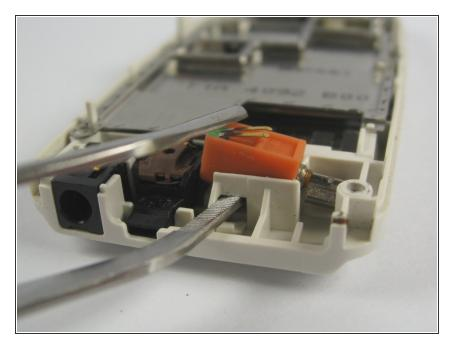
The vibrating unit is held in place by friction. Access the bottom of the unit and push upward to release it from the base.
