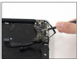
• Use the tip of a spudger to carefully flip up the retaining flap on the microphone cable ZIF socket.
