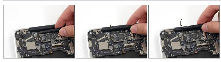
• Use the tip of a spudger to de-route the antenna cables from their notches in the logic board.
