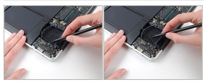
Gently de-route the camera cable from its notch on the I/O board and push it out of the way with the tip of a spudger.
