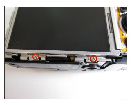
Remove the two screws that are attached directly below the screen with a #000 philips screw driver.
