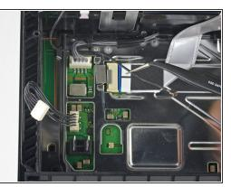
Use a pair of tweezers or your fingers to grab the antenna cable and move it out from the cable guides.
