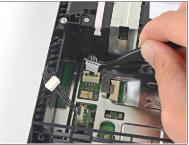
Use your fingers or a pair of tweezers to disconnect the optical drive cable from the motherboard.
