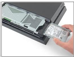
Pull the hard drive bracket out of the enclosure.
