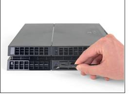
Use tweezers to remove the two stickers in the center of the back of the PS4 exposing two case screws.
