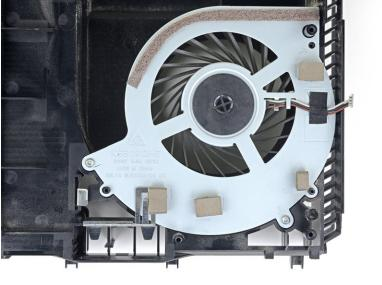
Remove the two 6.2 mm Phillips screws from the fan.
