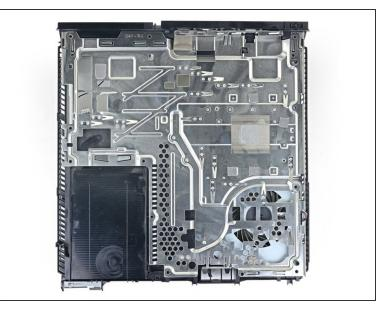
• Remove the three 6.2 mm Phillips screws from the lower EMI shield.
