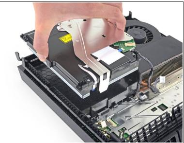
Lift the optical drive straight up and out of the PS4.
