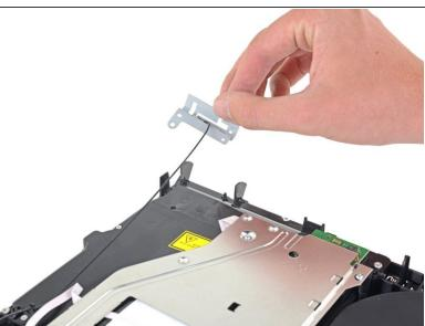
Remove the Wi-Fi antenna.
