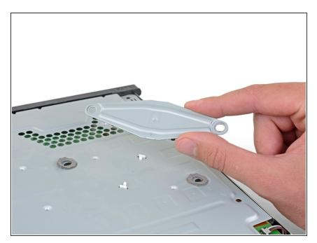
Remove the pressure plate.
