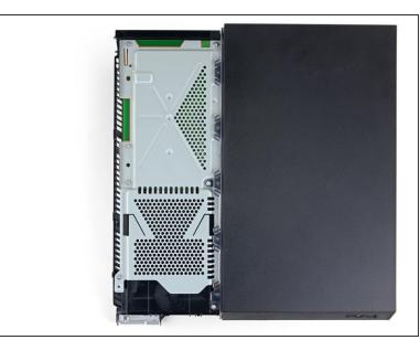
Remove the two 9.7 mm Torx screws securing the upper case.
