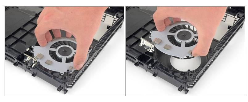
Lift the fan straight up out of the PS4 shell.
