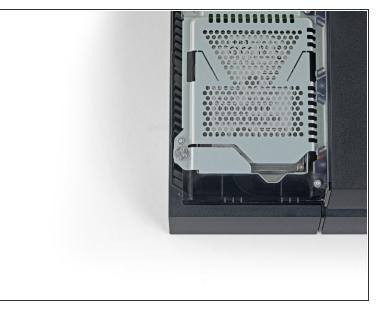
Use a Phillips screwdriver to remove the 6.5 mm screw securing the hard drive bracket to the enclosure.
