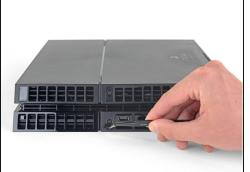
• Use <u>tweezers</u> to remove the two stickers in the center of the back of the PS4 exposing two case screws.
