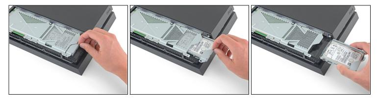
• Pull the hard drive bracket out of the enclosure.
