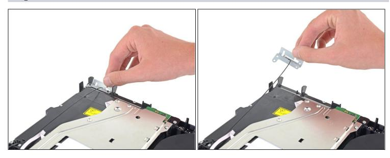
Remove the Wi-Fi antenna.
