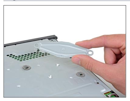
• Remove the pressure plate.
