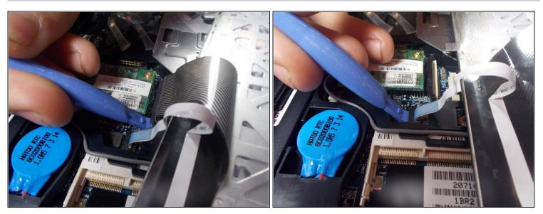
• Now with tweezers or a gentle prying apparatus gently pull the lock on the retaining clip up to release each ribbon cable. It is important to only pull up on the lock and not the entire clip.
