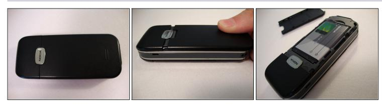
Press down on the grip on the back of the phone and slide the rear housing down towards the bottom of the phone.
