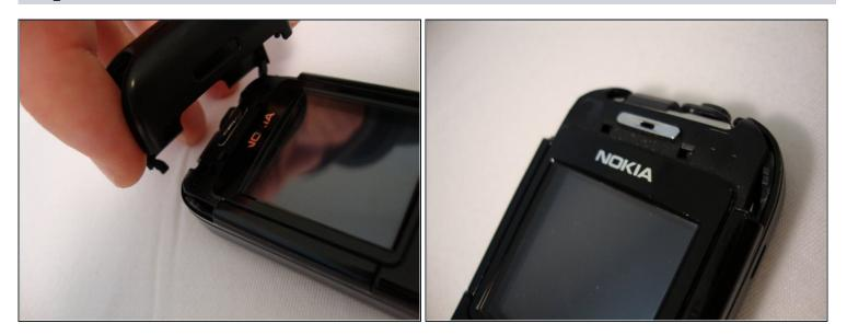
• After removing the top cover, turn the phone over so the screen is facing upwards.
