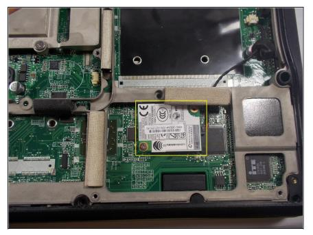
The internal modem will be located towards the bottom right of the laptop (highlighted with a yellow square).
