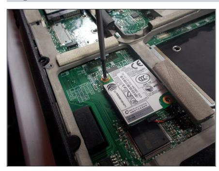
Using a Phillips #00 screwdriver, unscrew both of the screws that are holding the modem in place.
