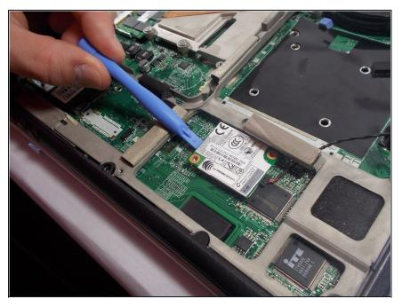
Carefully pry the modem as to not damage any of the surrounding components
