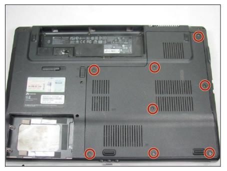
Remove the 8 screws from the back cover using the Phillips #00 screwdriver.
