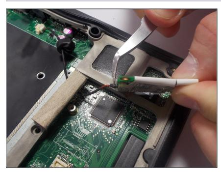
Using needle nose pliers, carefully detach the wire connecting the modem, by applying pressure to the black tabs away from the modem itself.
