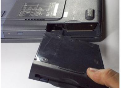
Slide tab in the direction of the arrow and pull out the floppy drive.
