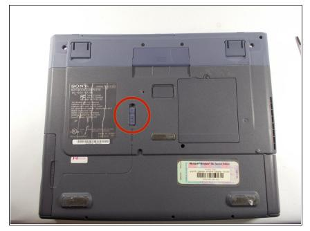
Locate the release tab on the bottom of the device.
