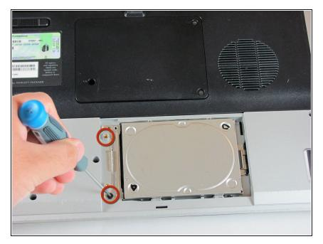
• Remove the two 5.0mm screws securing the hard drive bracket.
