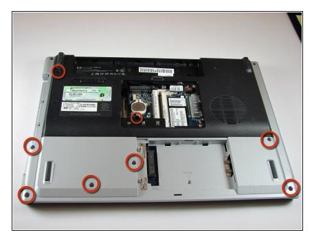
• Remove the eight 10mm screws securing the top cover to the laptop.
