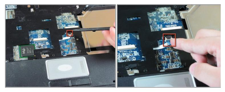
• Flip the computer over and disconnect the Touchpad Cable.
