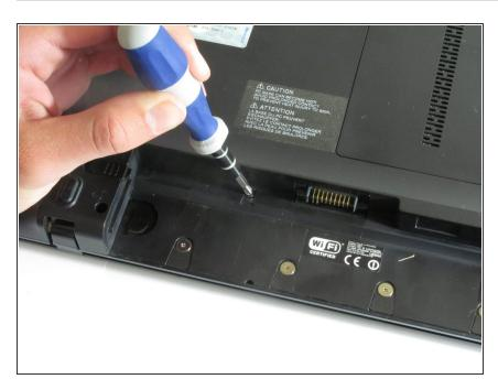
Using a #1 Phillips screwdriver, remove the 5.8 mm screw in the battery slot.
