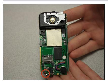
Locate the microphone on the back of the circuit board.
