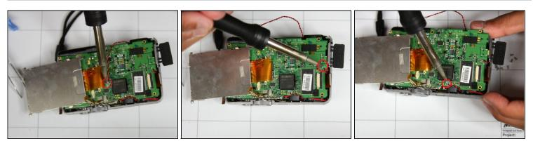
A Be very cautious when using a soldering iron for the next couple steps (they are on average 300 F)
