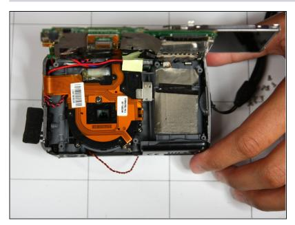
Slowly bend circuit board upwards (towards power button) until at 90 degree angle with remaining part of camera.
