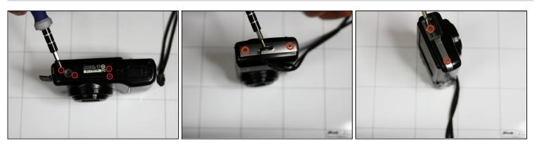
Remove 8 screws securing outside shell. Screw locations can be found in pictures
