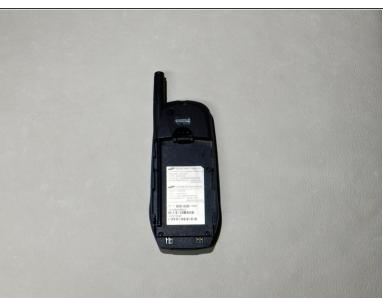
Slide the battery out from the battery compartment on the back of the phone.
