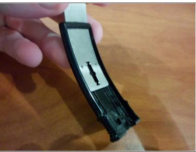
Turn the headphones so that the metal part of the headband located inside the outer covering can be seen.
