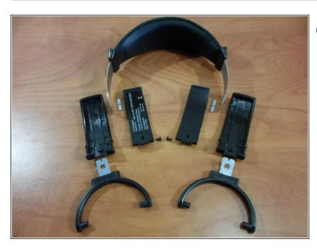
(i) All steps must be followed on both the left and right arms of the headband to free it completely from the outer coverings.
