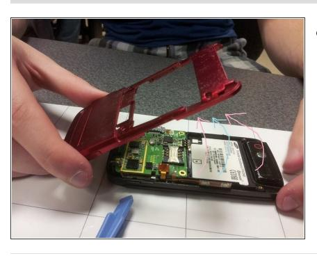
Finally, remove the back cover by gently lifting the case up, ensuring that nothing is still attached to the cover.
