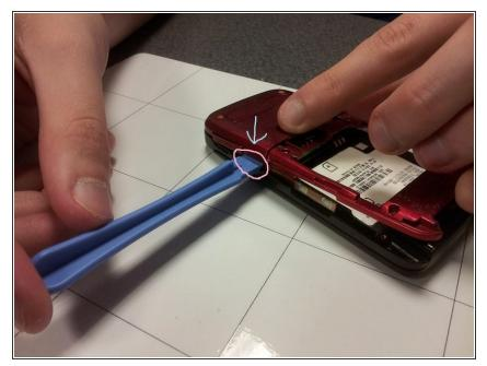
Continue using the prying tool to unlock the phone. If you hear a popping sound you know that you are on the right track. Be gentle as to not snap the screw-posts inside the case.
