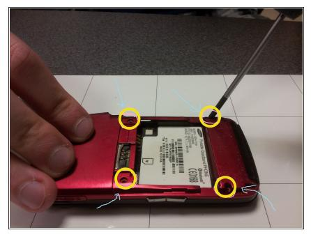
Place the phone face down on the table. Locate a Phillips head screwdriver. Begin by first removing the four screws that surround the upper area of the Samsung phone.
