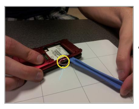
Next, remove the side button by prying open the the side of the phone with a prying tool. Insert the prying tool between the back cover and the remainder of the phone. Slide the prying tool to the left, creating a division between the cover and the phone.
