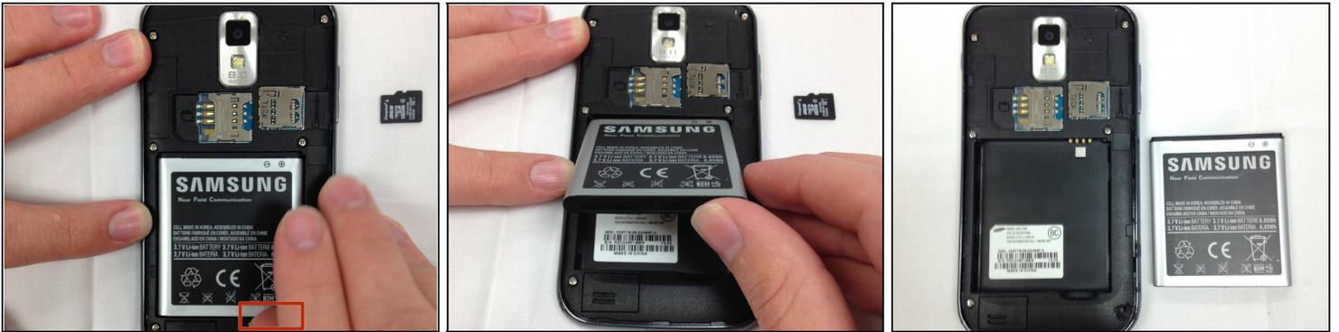
⚠ Turn off the phone before removing battery.
