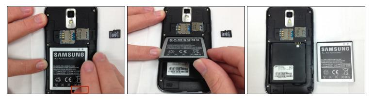
⚠ Turn off the phone before removing battery.
