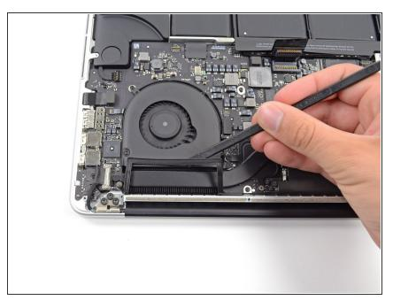
• Use the flat end of a spudger to lift the rubber heat sink cover up off the left fan.
