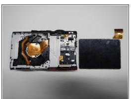
• Insert the flat side of the spudger tool carefully on the top of the LCD screen and lift the screen free
