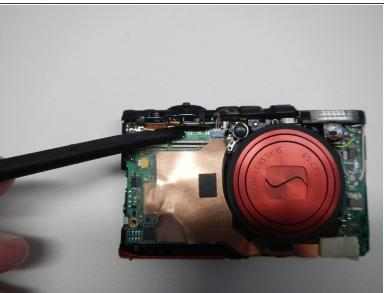
Disconnect the copper ribbon next to the blue port on the motherboard
