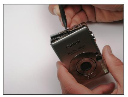
Pull the lanyard mount off of the camera using a spudger or your fingers.
