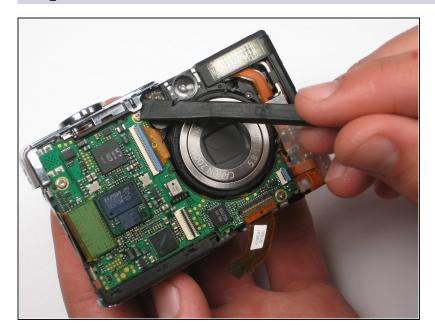
Lift up the metallic-colored clip with the spudger to remove the shutter panel.
