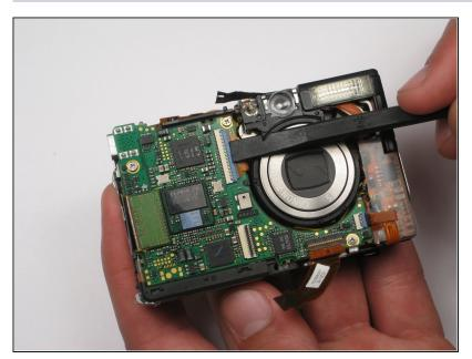
• Use the spudger or your finger to release the orange ribbon from the logic board.
