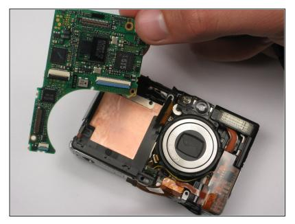
• Remove the detached logic board from the camera.
