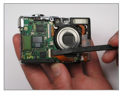
Remove the LCD cable by gently prying the hinge open with a spudger or your finger.
