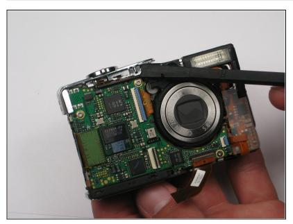
Remove the shutter panel with the spudger, now that the clip is released.
