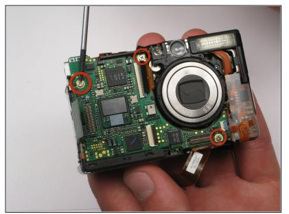
Use the screwdriver to remove the three screws on the logic board. Take note that the bottom right screw is shorter than the other two.
