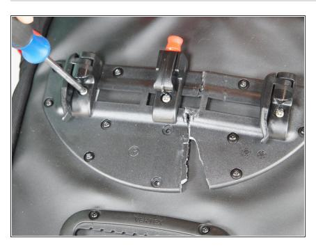
To remove clip bracket, first remove all 3 clips using the #2 screwdriver or hand drill (Make sure to put clips and their screws and anchor plates in a safe place as to not misplace any such as a Ziploc bag).
