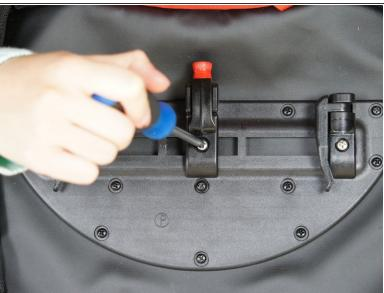
Remove old clip. Take new clip bracket and unscrew and remove middle clip.
