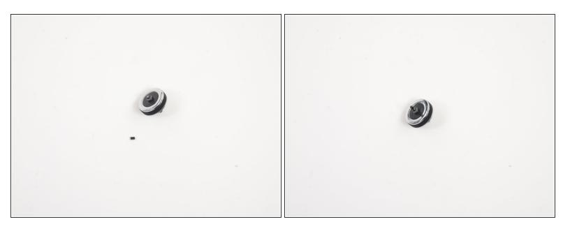
Glue broken axle piece back onto the scroll wheel.
