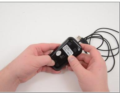
Slide the tab on the bottom of the mouse to release the top panel.
