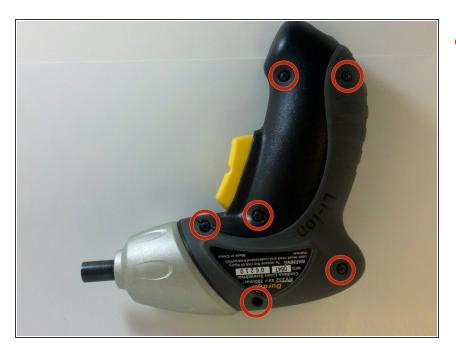
Remove the six 13 mm casing screws with the #0 Phillips screwdriver.
