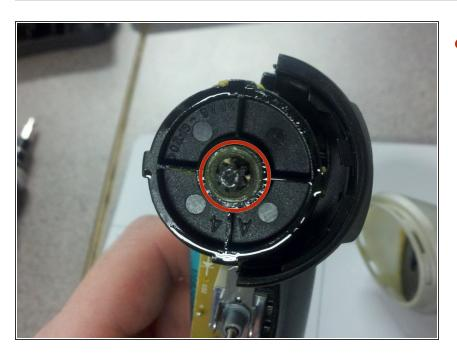
Apply a dab of grease to the end of the drill motor coupler.
