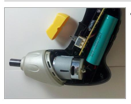
Insert new bit chuck assembly into the drill casing.
