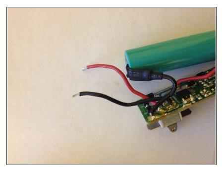
Strip the ends of the wires clean with the wire cutters. Strip the wire insulation 1/4" from the end of the wire.
