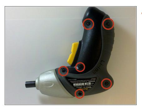
Remove the six 13 mm case screws with philips #0 screwdriver.
