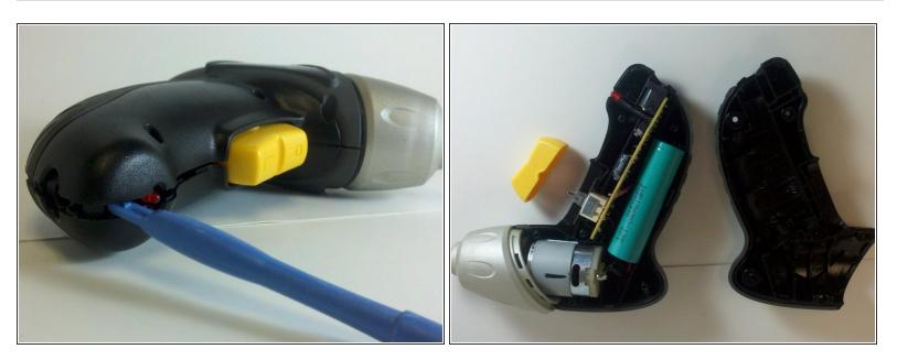
• Use the plastic separating tool to separate the casing halves of the cordless screwdriver.
