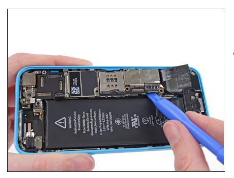
Use a plastic opening tool to gently lift the lower end of the logic board up from the rear case enough for you to grab it with your fingers.
