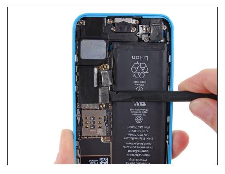
Disconnect the Lightning connector ribbon cable from its socket on the logic board.
