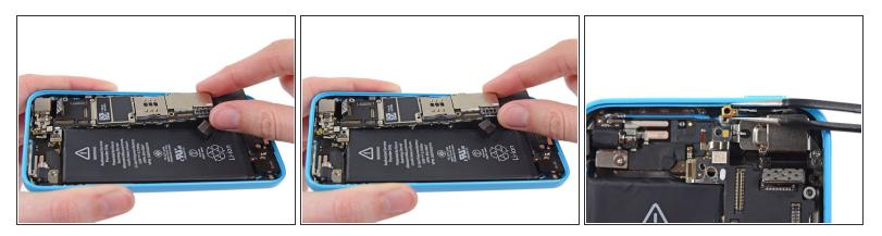
• Pull the logic board away from the rear-facing camera just enough to expose the gold contact cap under the top end of the board.
