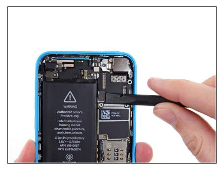
Use the flat end of a spudger to disconnect the audio control cable connector from its socket on the logic board.
