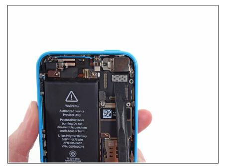
Disconnect the rear facing camera cable connector from its socket on the logic board.
