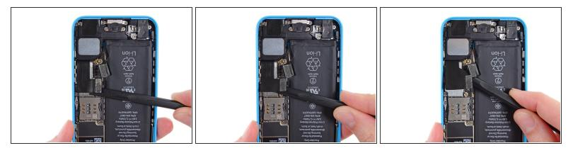
The Lightning connector cable is lightly adhered to a shield on the logic board. Use the flat end of a spudger to gently peel the cable up.
