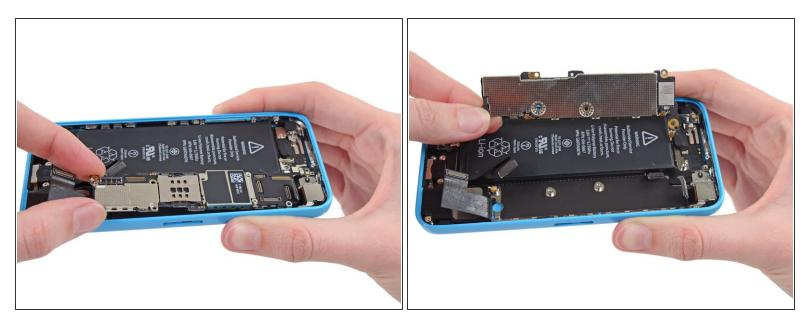
• Flip the logic board up toward the volume control buttons to expose the antenna connector.
