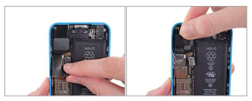
• Fold the cable up out of the way of the logic board.
