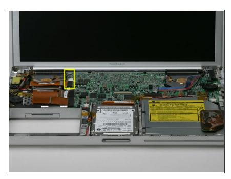
Disconnect the Orange ribbon cable, inverter cable, and fan cable from the logic board.
