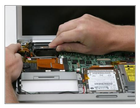
Lift the fan and attached black tape out of the computer, lifting from the front edge.
