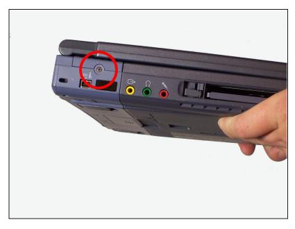
Use your Philips #00 screwdriver to unscrew the small screw counterclockwise.
