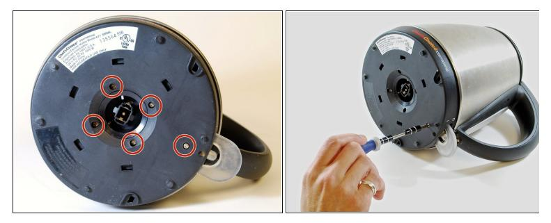
• Remove the five 3/8" screws from the base of the kettle using a Phillips #1 screwdriver.
