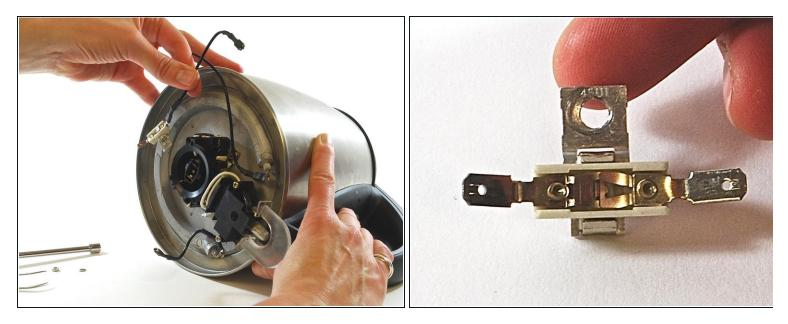
• Using your hands, grasp the wire that is still connected to the power supply. Carefully lift the power supply off the threaded stud to which it was coupled.
