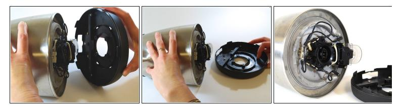
• Using your hands, remove the kettle base by sliding it over the switch.
