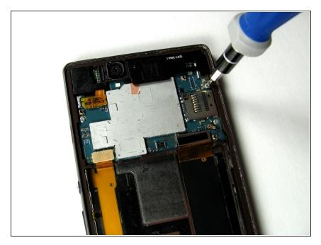
Remove the one 3 mm screw with the Phillips #000 screwdriver. The screw is located at the top right corner of the motherboard. The motherboard is the green/silver circuit board at the top of the phone.
