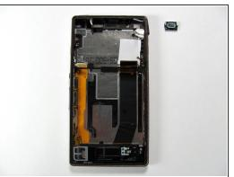
Gently pry the ear speaker out of its position, making sure to keep the tool beneath the adhesive attached to the ear speaker.
