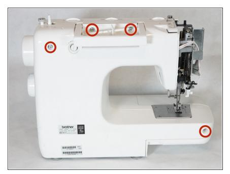
Remove the two 14mm Phillips #2 screws and two 22mm Phillips #2 screws that secure the rear casing.
