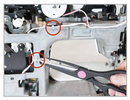
• Using scissors, clip the two zip ties securing the lightbulb wire.
