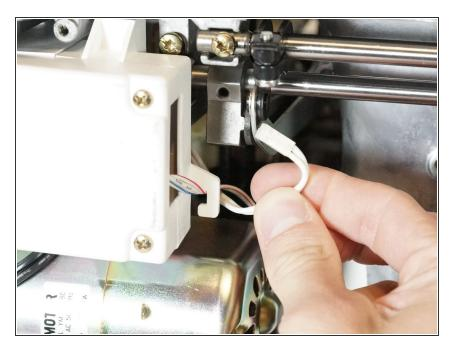
• Move the wire out from under the plastic hook.
