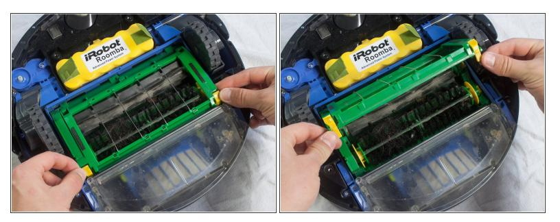
Pinch the yellow tabs on the sides of the brush cage and lift up to open.
