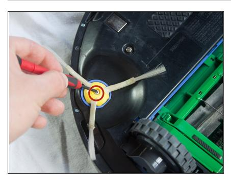
While holding the side brush in place, use a Phillips #1 screwdriver to remove the 4.5mm screw from the center of the brush.
