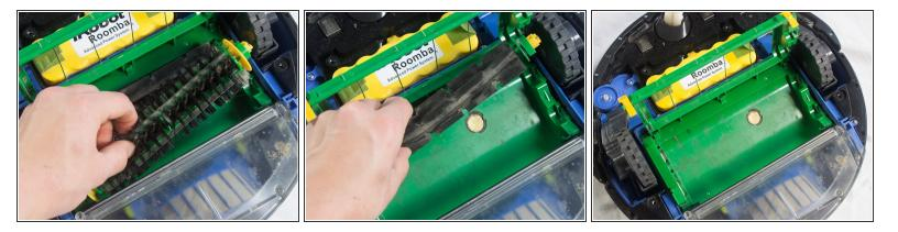
Grab each brush and lift upwards to remove.
