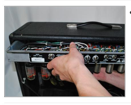
Repeat steps 6 through 1 in reverse order to rebuild your amp! Ensure to always use only one hand in the amp and to keep your tubes safe.
