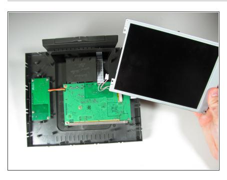
Remove the display assembly from the device.
