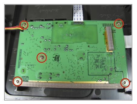
Remove the five 7mm Torx T6 screws.
