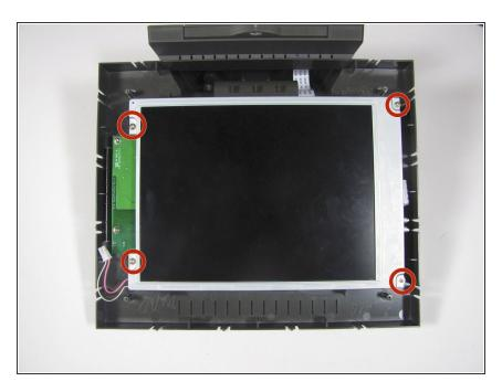
Remove the four 7mm Torx T6 screws.
