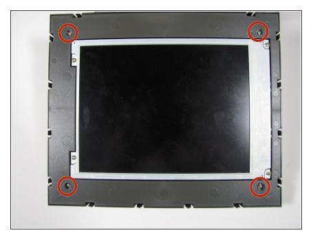
Remove the four 7mm Torx T6 screws.
