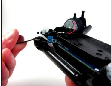
Gently detach the touchpad ribbon connected to the motherboard using the blunt forceps. The
