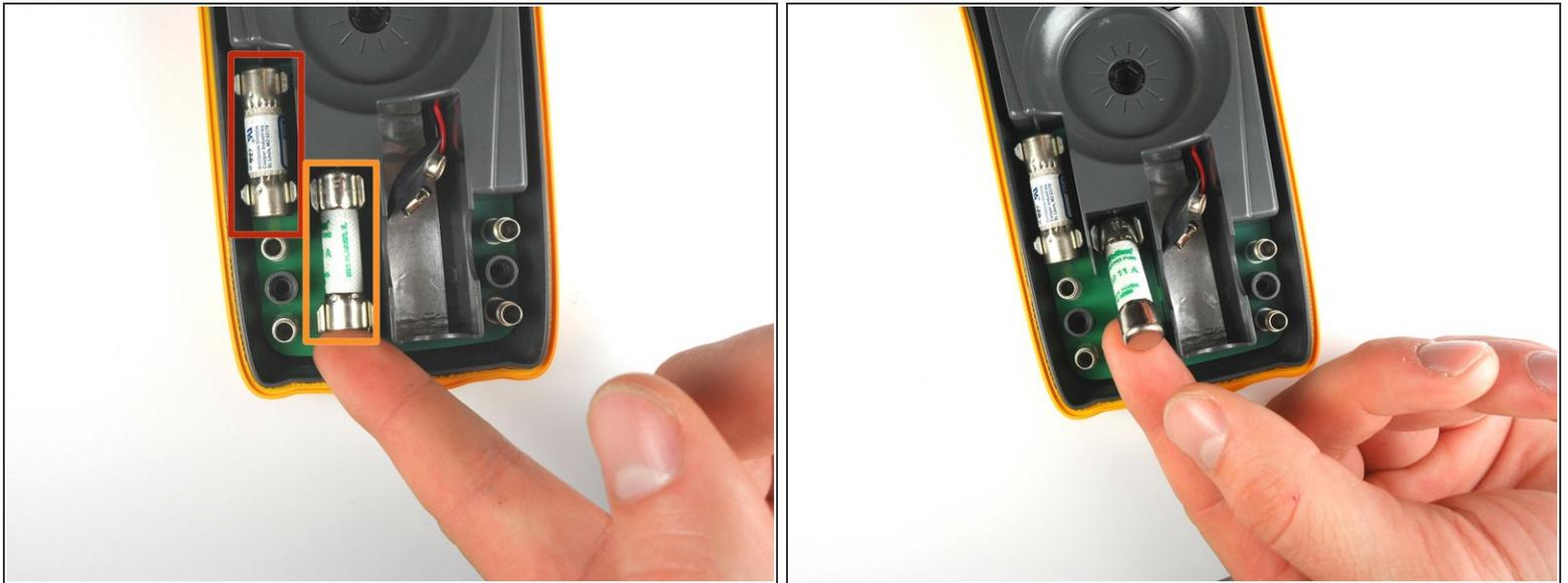
**⚠** Replace a fuse only with a fuse identical in type, voltage rating, and current rating as specified by the back panel fuse rating label or the [Fluke 77 Series III Service Manual](#). Inserting the wrong replacement fuse could create a fire hazard.
