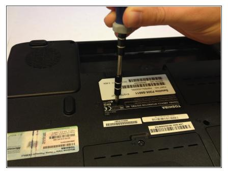
• Remove the 8mm Phillips #1 screw that holds the disk drive in place.
