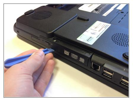
• Use a plastic opening tool to pry out the disk drive.
