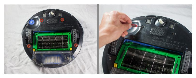
• Using a Phillips #2 screwdriver, remove the captive screws that hold the bottom plate in place.
