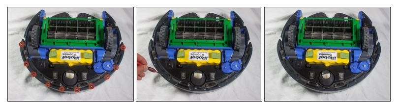
With a Phillips #1 screwdriver, remove the ten 12mm screws located along the bottom of the bumper.
